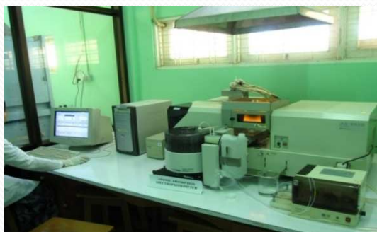
Atomic absorption spectrophotometer AA 6650
