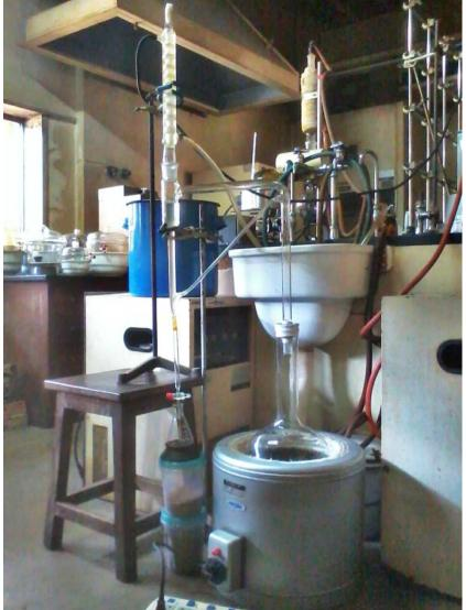
Hydrodistillation apparatus for extraction of essential oil
